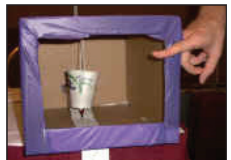
Left: A modified Model Seismograph made by John Lahr. The tin can is suspended from a loop of wire that only allows it to move in one direction. A marking pen is pushed through a hole in the bottom of a can, which is then filled half way with small pebbles.
